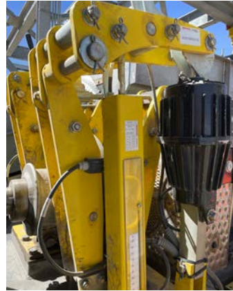
DT 315 FEM, DS 160 FEA, DS 230 FEM and DT 250 FEA as emergency and holding brakes
