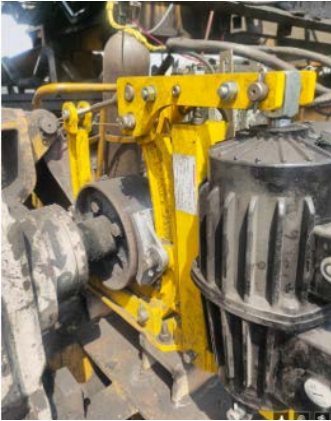
DT 315 FEM, DS 160 FEA, DS 230 FEM and DT 250 FEA as emergency and holding brakes
