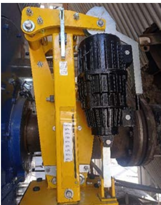
DS 370 FEA as stopping and holding brake
