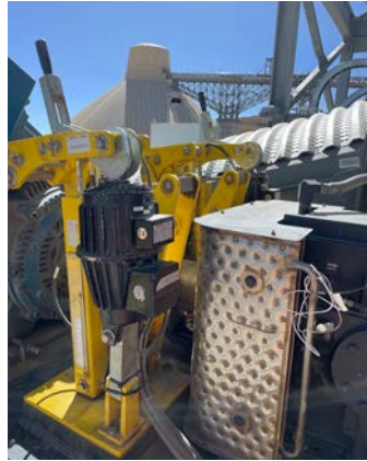
DT 315 FEM, DS 160 FEA, DS 230 FEM and DT 250 FEA as emergency and holding brakes
